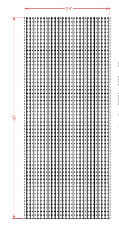
NOTE: LOOSE LAID CROSSGRIP PAD IS SUITABLE FOR ALL LOW WIND AREAS (NO WELDING REQUIRED)
