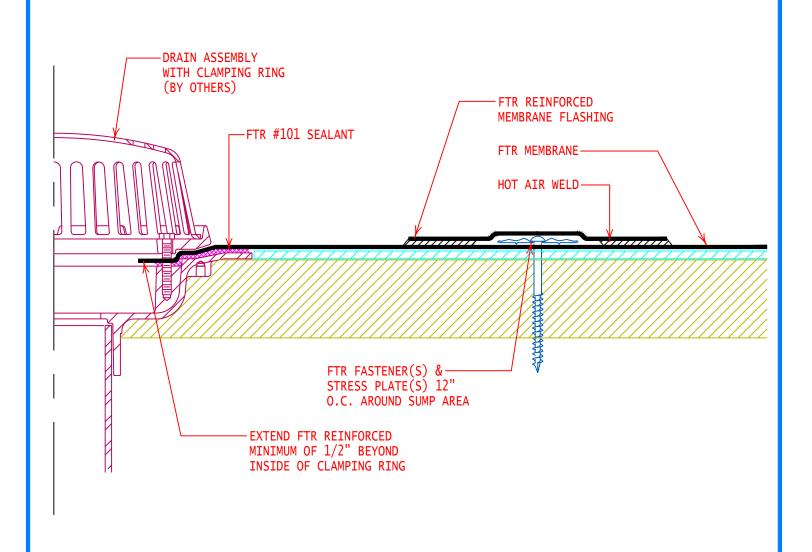
NOTE: CENTER THE DRAIN IN THE MIDDLE OF THE FIELD SHEET. MINIMUM WIDTH OF FIELD SHEET IS 74" AND SECURE AT 12" FROM DRAIN CENTER.
