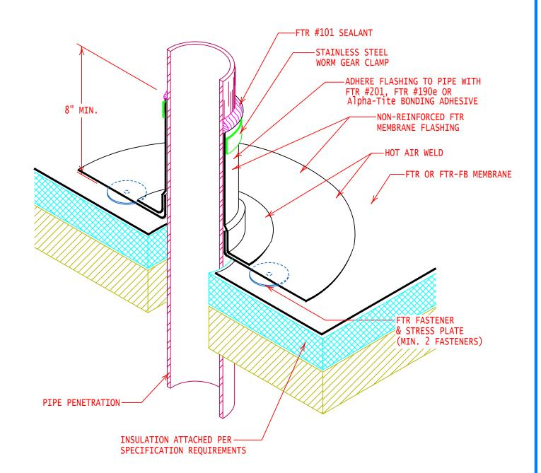
FOR PENETRATIONS LESS THAN OR EQUAL TO 6 IN, ONLY TWO (2) PLATES AND FASTENERS ARE REQUIRED. FOR PENETRATIONS GREATER THAN 6 IN, FOUR (4) FASTENERS AND PLATES ARE REQUIRED.
