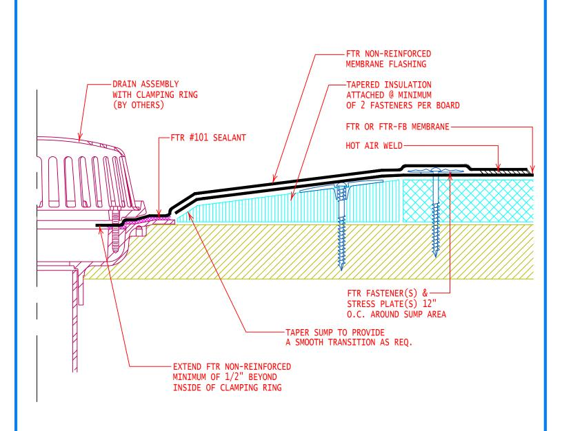
NOTE: USE TAPERED ROOF INSULATION (EDGE STRIPS) TO CREATE DRAIN SUMP. IF TOTAL INSULATION THICKNESS IS LESS THAN OR EQUAL TO 1 1/2 IN., TAPER 12 IN. FROM THE DRAIN CENTER. IF TOTAL INSULATION THICKNESS IS GREATER THAN 1 1/2 IN., TAPER 18 IN. FROM DRAIN CENTER.
