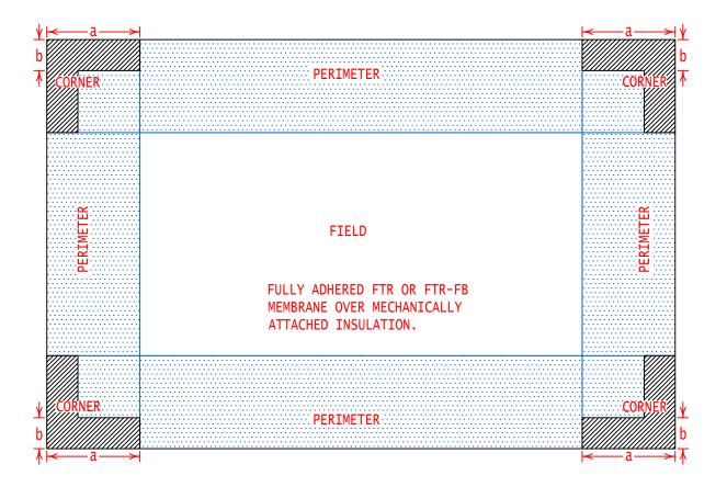
FOR BUILDING HEIGHTS UNDER 60FT, PERIMETER (DIMENSION "a") AND CORNER (DIMENSION "b") ARE DETERMINED AS 60% OF THE BUILDING HEIGHT FOR THE PERIMETER AND 20% OF THE HEIGHT FOR THE CORNER. (SEE DETAILS FTR-ASCE7a THROUGH ASCE7d FOR MORE DETAILED INFORMATION.)
